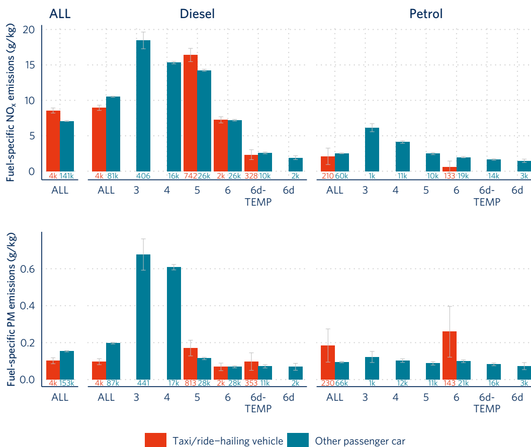
Figure 22. Mean fuel-specific NO x and PM emissions (g/kg) from Brussels taxis and ride-hailing vehicles and other passenger cars by fuel type and emissions standard. The number of measurements is presented under each bar. Whiskers represent the 95% confidence interval of the mean.
