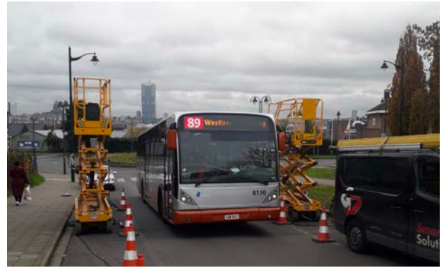
Figure 3. Remote sensing emissions testing of buses at the BRU0018 site on Boulevard Jules Graindor.
